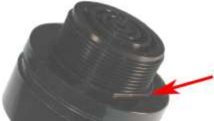
For a vast majority of applications, the locking flats do not need to be used. If the knurled nut (not shown) is properly tightened, the alarm will not move in the application. However, for some high end applications with a lot of vibration (such as aerospace), the locking flats would help to ensure that the alarm will not rotate within the panel which could end up putting pressure on the wiring connections to the terminals of the alarm.
